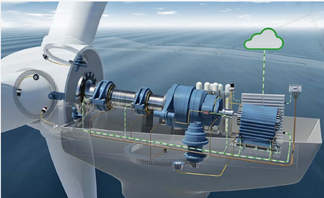
Sensitive: sensors in the drivetrain report condition information of wind turbines in real time
