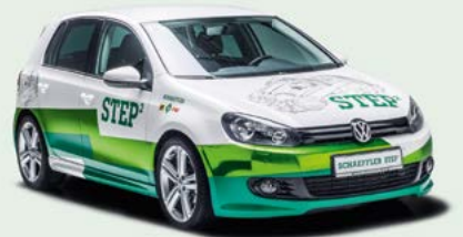
Concept vehicle in Golf guise. With wheel hub motors and a two-speed powershift transmission. The variable gear ratio improves fuel economy by 6%.
